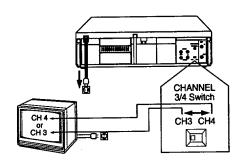
Set the TV to channel 3 or 4, whichever channel the CH3/CH4 switch on the back of the TV is set to.
